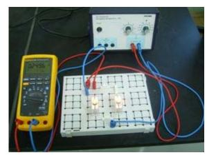
• As you increase the potential difference, in 1.0V up to 4.0V, measure and record the voltage and current.
